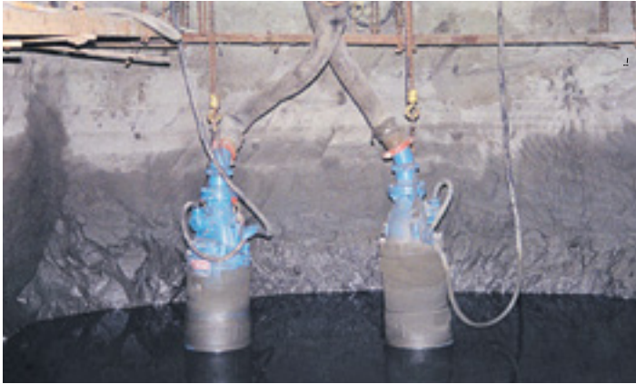
: Slimline Pumps - Pump diameter less than 15"
